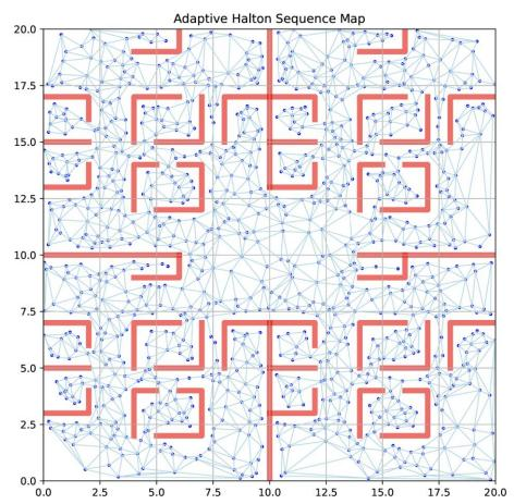
The Adaptive Halton Sequence adjusts point density based on the distribution of obstacles. It assigns lower point density in open areas and higher point density in regions with dense obstacles.
